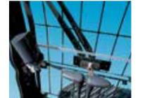
Windshield wiper motor positioned for ample foot room and a clear view.
