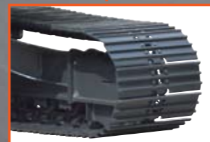
Durable forged steel shoe
