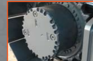
Stronger casing for travel motor
